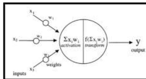
Figure 3. Artificial neural network model
