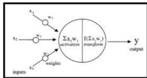
Figure 3. Artificial neural network model
